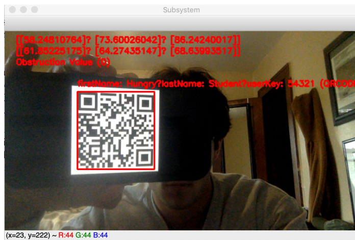
Figure 8. QR Code Detection, Obstruction Detection on a Video Stream
