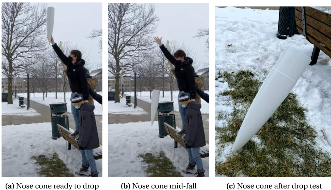
Figure 86: Photos of the nose cone tip-first drop test
