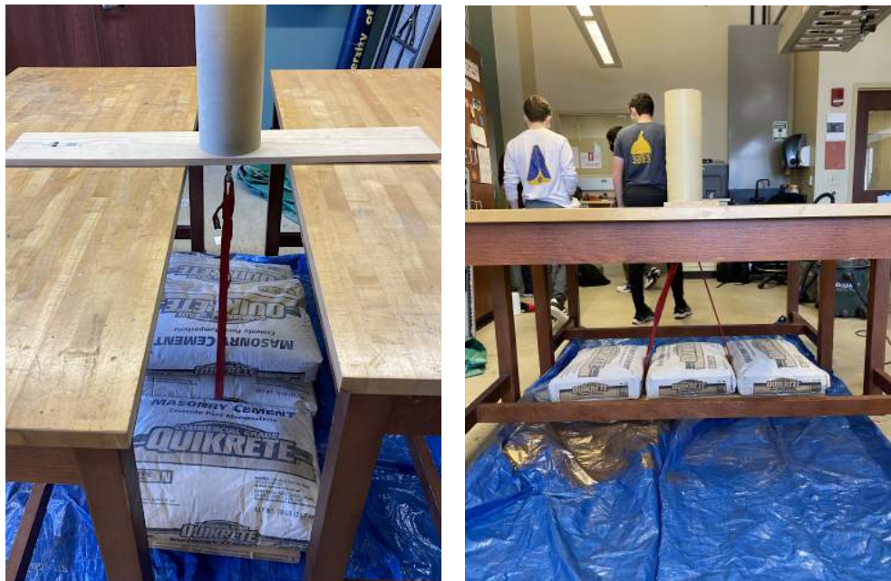
Figure 83: Bulkhead assembly strength test with 310 lb suspended from the test article
