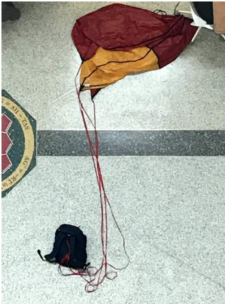
Figure 96: Image taken after completion of balcony drop testing of the main parachute.
