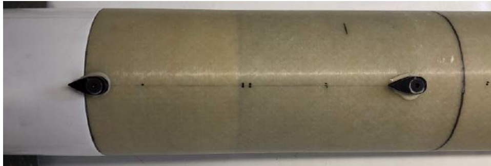
Figure 19: The two rail buttons used to control the launch angle fastened to the fin can
