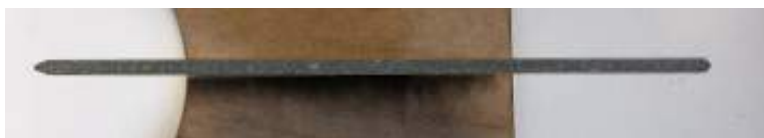
Figure 9: Airfoil cross-section of a fin with LE on the right and TE on the left
