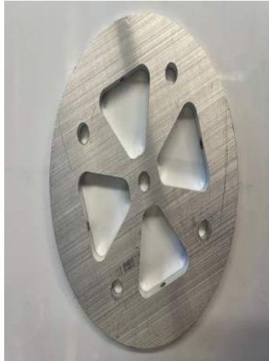
Figure 25: ACS Aluminum bulkhead.
