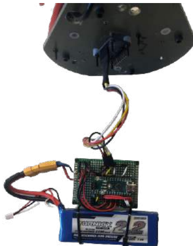
Figure 57: Electronic configuration of Arduino controlling the servo motors.
