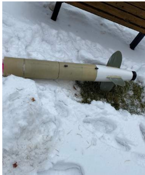
(b) Fin can assembly after drop test
