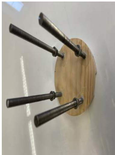
Figure 26: Threaded rods mounted to wooden bulkhead.
