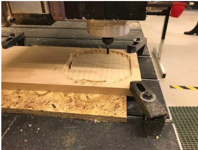
Figure 24: Manufacturing of the twist to lock mechanism alignment ring on the Techno Router
