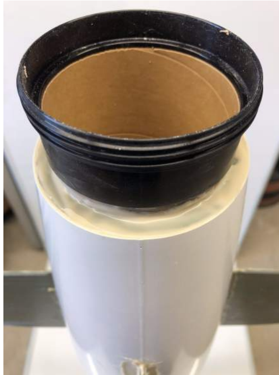
Figure 17: Centering ring at the boattail aft opening in the finished motor retention assembly
