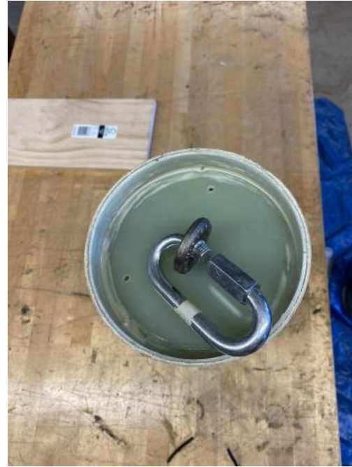
(b) Bottom view of the test article with quicklink attached to eyebolt
