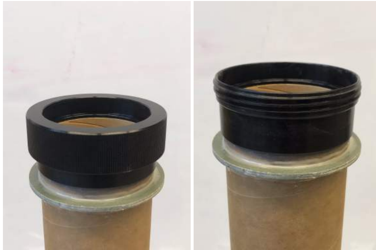
Figure 16: Motor retainer secured to the motor mount tube
