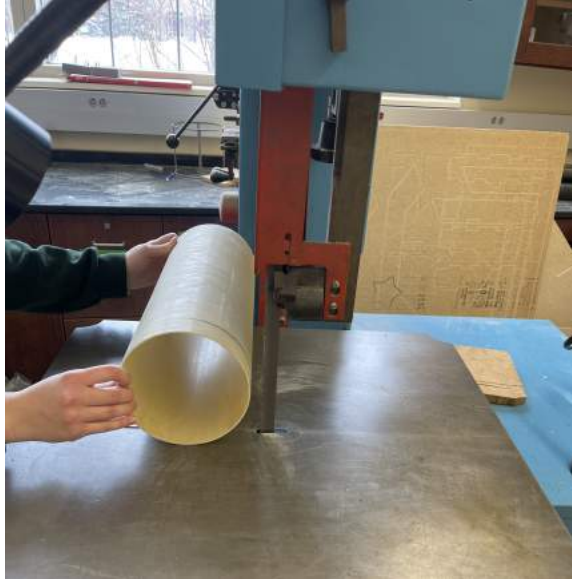
Figure 13: Alignment of the body tube to be cut on the bandsaw.
