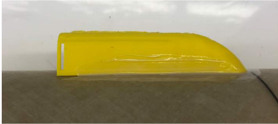
Figure 12: Side view of the camera shroud epoxied to the payload tube
