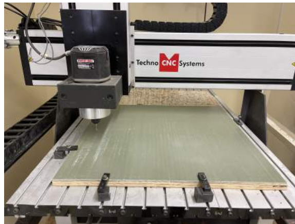
Figure 14: The \frac{1}{8} fiberglass clamped onto the CNC router bed.
