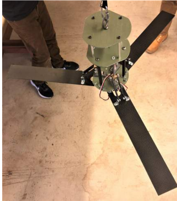
Figure 58: Payload legs in landing configuration.
