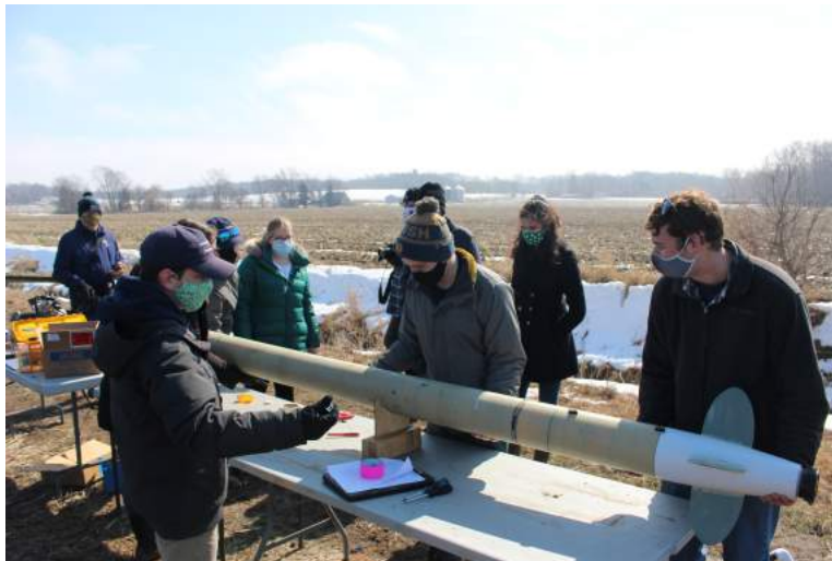
Figure 78: CG Location and Stability Check
