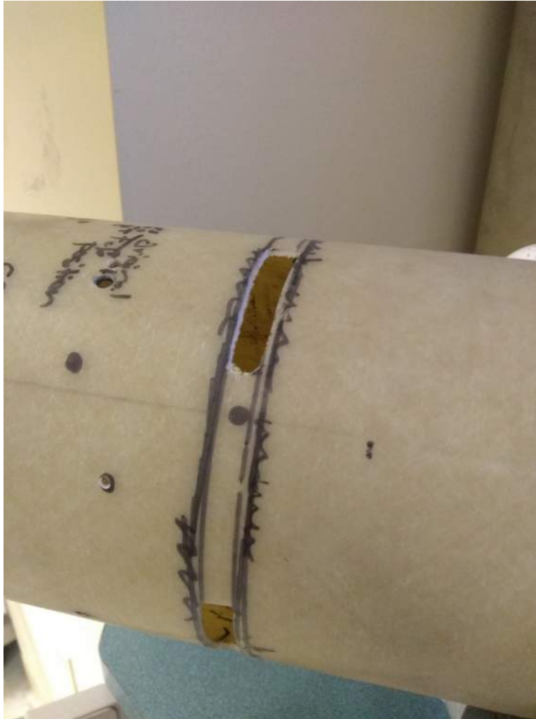
Figure 29: ACS Fin Can Tab Interfaces
