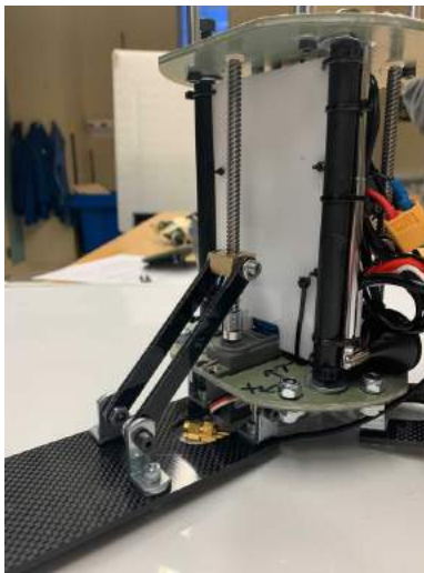
Figure 55: PLS legs subsystem: servo motor, threaded rod, bronze shaft, and arms
