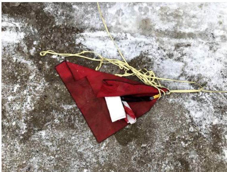
Figure 94: Undamaged Nose Parachute and Harness After Ground Testing
