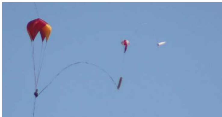
Figure 64: In-Flight Photos of CRAS-S Deployment Off-Nominal Event
