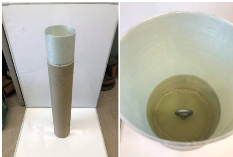
Figure 15: An assembled coupler (left) and the interior with the bulkhead attached (right)
