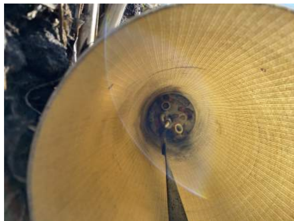
(b) 1 Failed Charge
