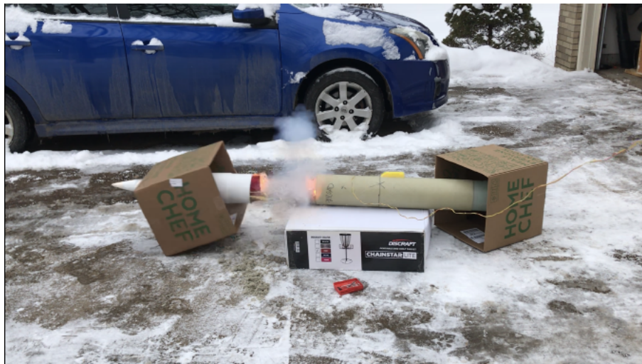
Figure 93: CRAS-S black powder ground testing
