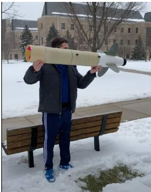
(a) Fin can assembly ready to drop
