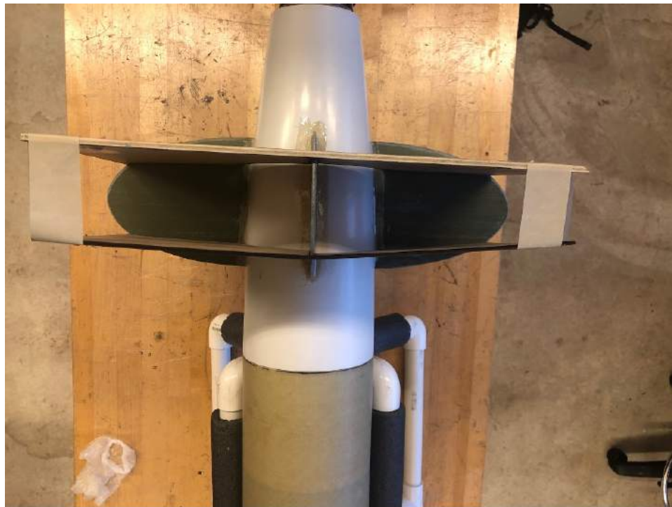
Figure 18: The epoxied fins held in place by the fin alignment jig
